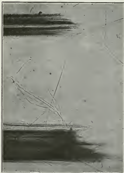
Break in fibre from Casper mountain, Wyoming, U.S.A. Magnified 150 diameters.
